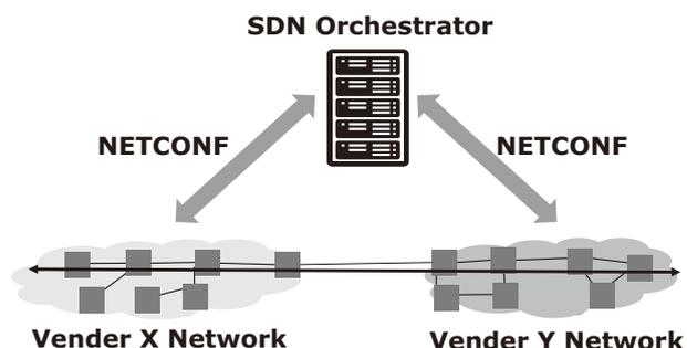
Fig. 1 Monitoring and control of devices using NETCONF.
