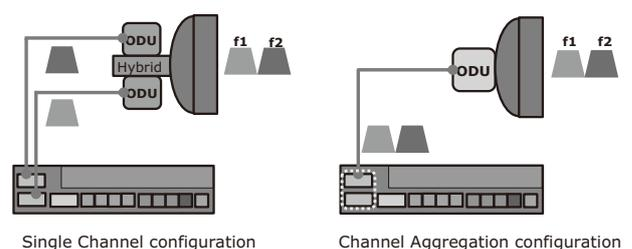
Fig. 2 Channel aggregation configuration.
