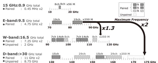
Fig. 5 Frequency relationship between microwave-band (15 GHz), E-band, W-band, and D-band.
