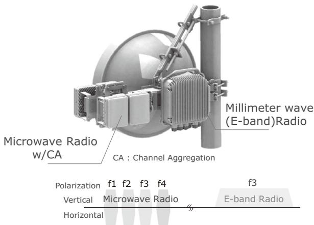
Fig. 3 Multiband configuration.
