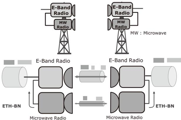
Fig. 4 Example of multiband aggregation configuration.
