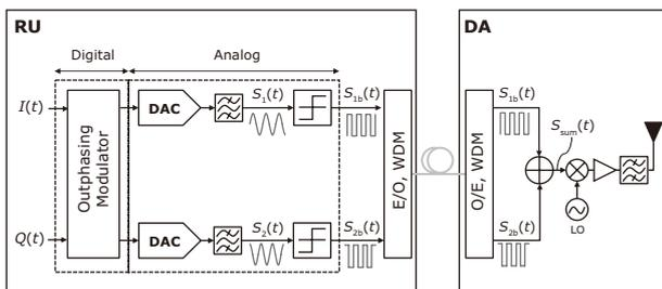
Fig. 5 Block diagram of proposed RoF system.
