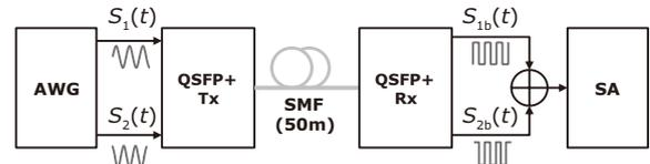
Fig. 6 Experimental setup for evaluating proposed RoF system.
