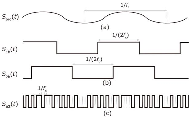
Fig. 4 Waveforms of (a)  $S_{orig}(t)$ , (b) pair of  $S_{1b}(t)$  and  $S_{2b}(t)$ , and (c) conventional  $S_{\Delta\Sigma}(t)$ .
