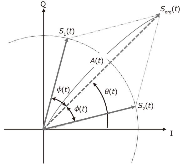
Fig. 3 Principle of outphasing with vector separation.
