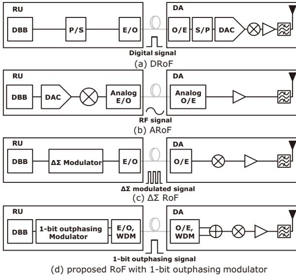
DBB: digital baseband, P/S: parallel-to-serial converter, S/P: serial-to-parallel converter, WDM: wavelength division multiplexing
