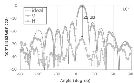
Fig. 11 Azimuth beam patterns and cross-polarization isolation of the 8×2 phased array module at a beam angle of 0° and 10°.
