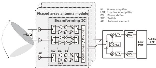
Fig. 1 Phased-array transceiver configuration.
