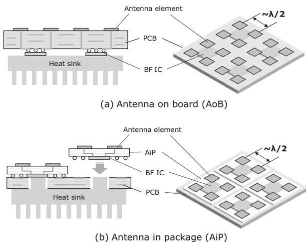
**Fig. 4** Implementation styles of front-end modules.
