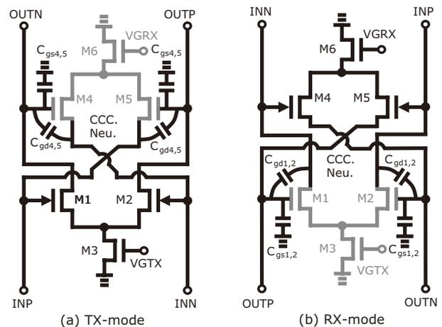
Fig. 3 Circuit diagram of bi-directional amplifier.
