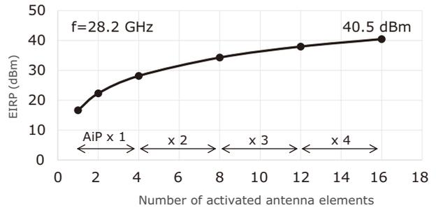
Fig. 9 Measured EIRP of developed 8×2 phased array module.
