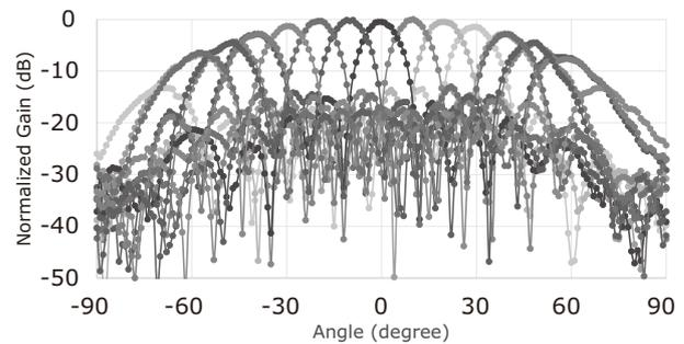
Fig. 10 Measured azimuth beam patterns of the 8×2 phased array module.
