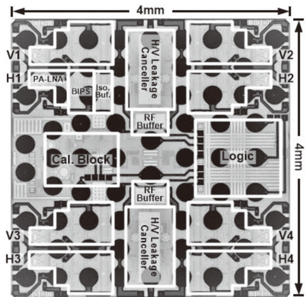
**Fig. 5** 28 GHz band 8-element BFIC.
