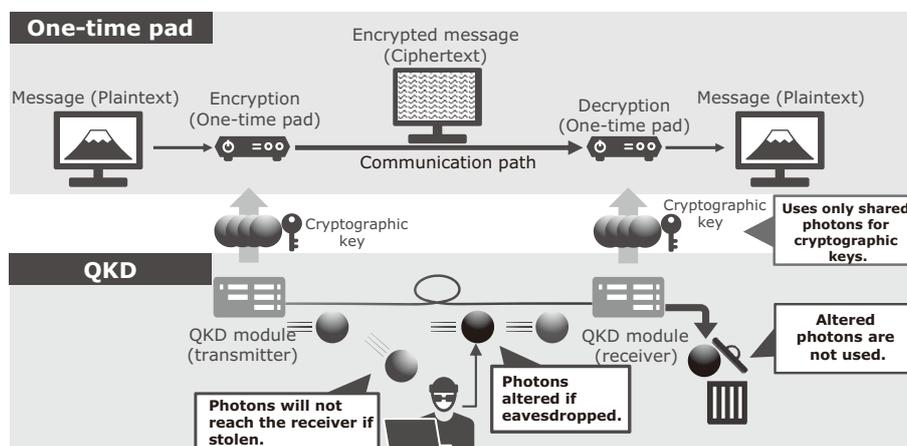
Fig. 1 Outline of how quantum cryptography works.
