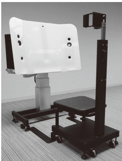
Photo 3D facial contour measurement system.
