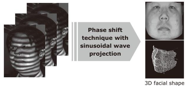
Fig. 1 Measurement example of 3D facial contours.
