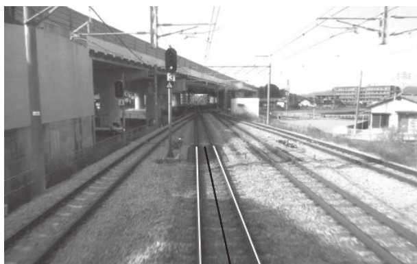
(a) Rail detection White lines: rails; black line: center of track.
