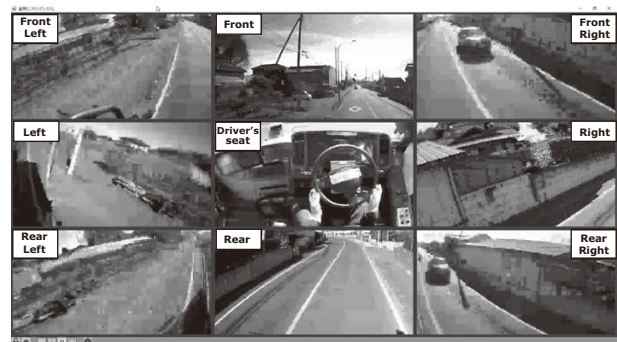
Photo 2 Examples of surveillance screens from the self-driving bus demonstration test on public roads.
