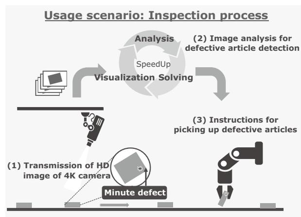
Fig. 4 Usage scenario: Inspection process.
