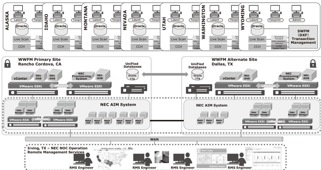
Fig. 2 Architecture of the three-tiered WIN system.
