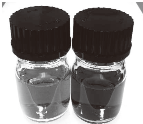
Fig. 3 Separated liquids of semiconducting CNT (Left) and metallic CNT (Right) collected after separation.
