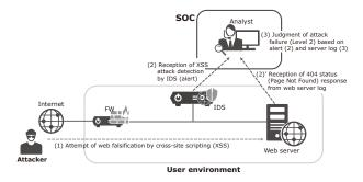
Fig. 5 Example of efficient judgment made by combination of multiple logs.
