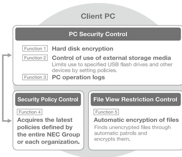
Fig. 7 Overview of information leakage prevention system.
