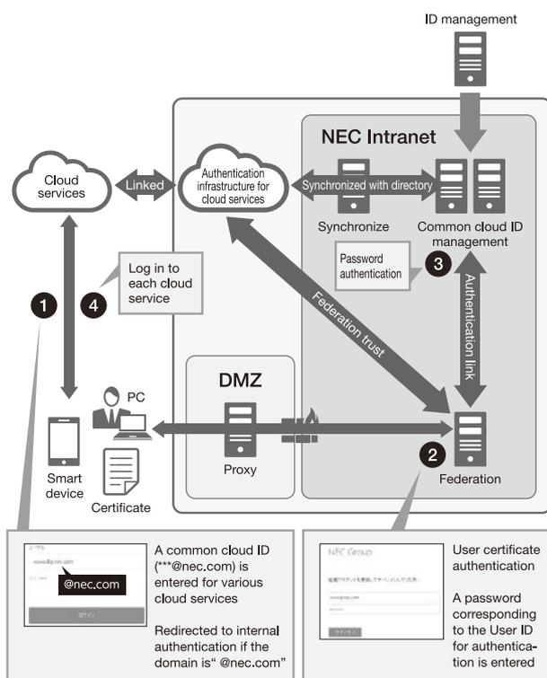
Fig. 5 Cloud authentication linkage.
