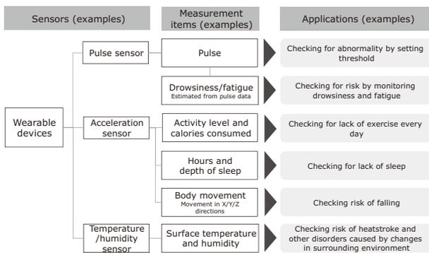
Fig.1 Examples of information that can be obtained by wearable devices.
