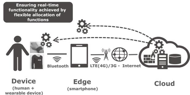
Fig. 5 Allocation of functions in edge devices.
