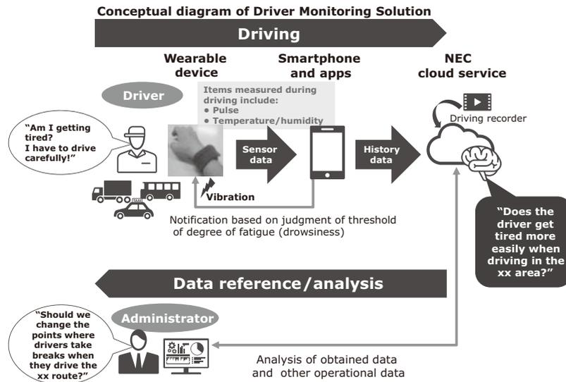
Fig. 3 Conceptual diagram of Driver Monitoring Solution.
