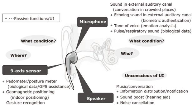
Fig. 6 Features of a hearable device.
