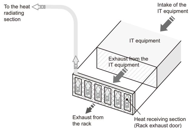
Fig. 5 Phase change cooling of a rack.
