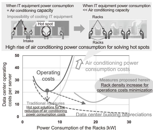
Fig. 2 Power consumption and operating cost of racks.
