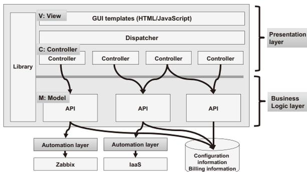
Fig. 2 Architecture of the self-service portal.
