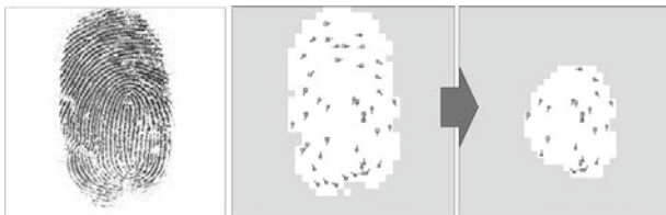
Fig. 5 Reducing computational cost by minutia pruning.
