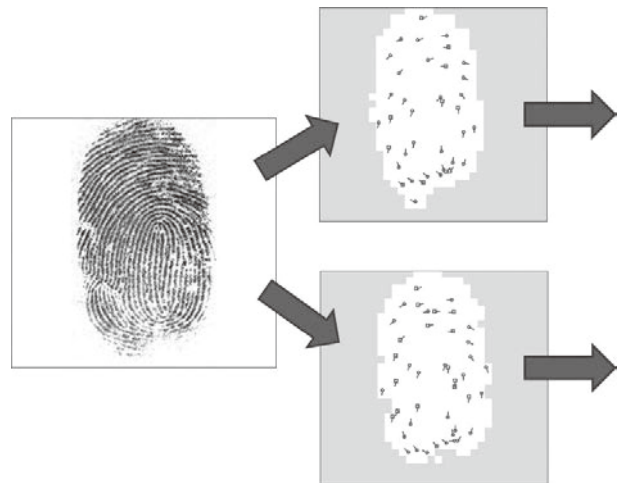
Fig. 6 Risk reduction by adopting more than two minutia extraction methods.
