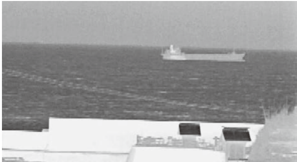
Fig. 6 IR camera image of a ship at 2.5 km distance.
