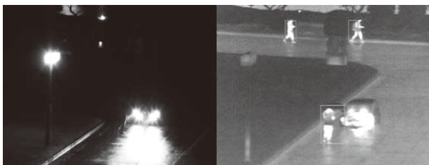
Fig. 7 Comparison of visible-light camera (left) and IR camera (right).
