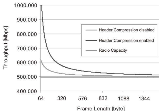
Fig. 4 Effects of header compression.
