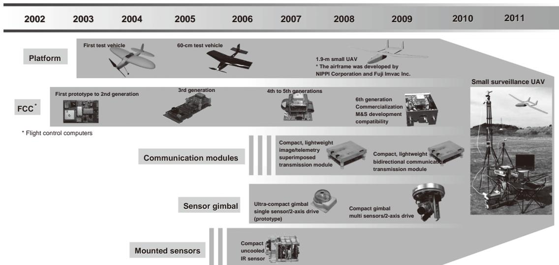
Fig.1 History of the development of technologies associated with the small UAV system.
