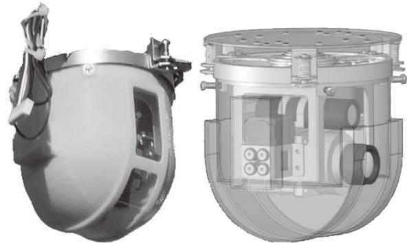
Fig. 2 External view and internal structure of the sensor gimbal.
