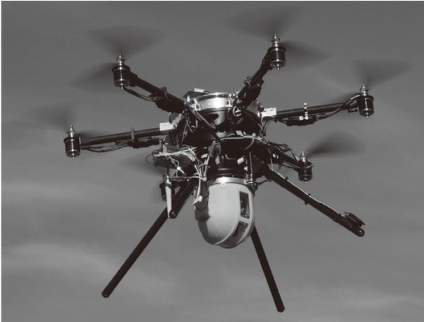
Photo 3 Sensor gimbal mounted on a multi-rotor helicopter.
