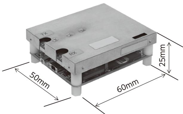
Photo 2 External view of the compact image transmission module.
