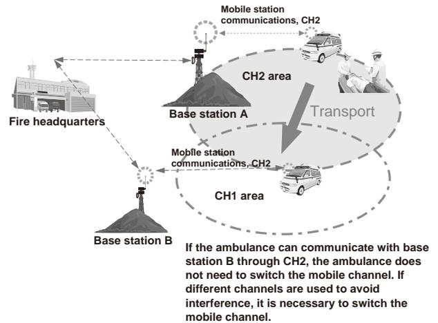
Fig. 5 Channel switching per area.
