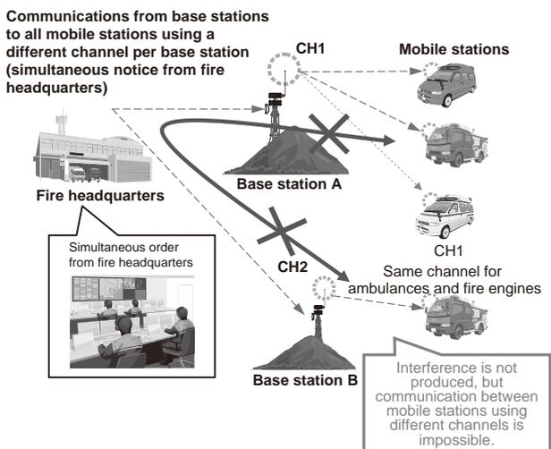
Fig. 4 Channel switching per base station.
