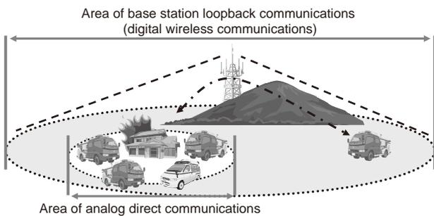
Fig. 1 Comparison of communication area between analog wireless and digital wireless communications.
