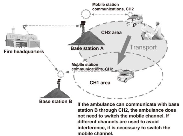
Fig. 5 Channel switching per area.
