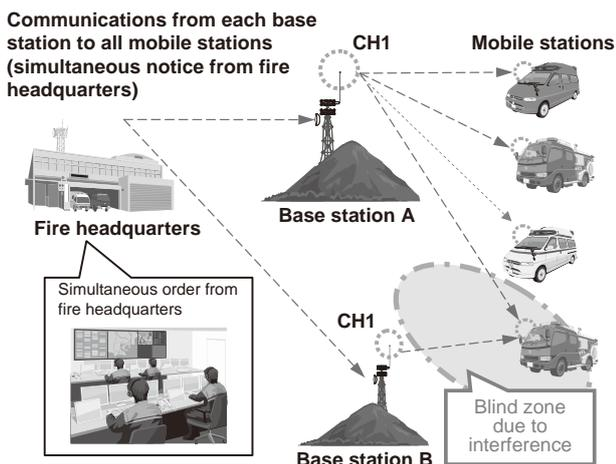
Fig. 3 Radio interference caused by simultaneous notice.
