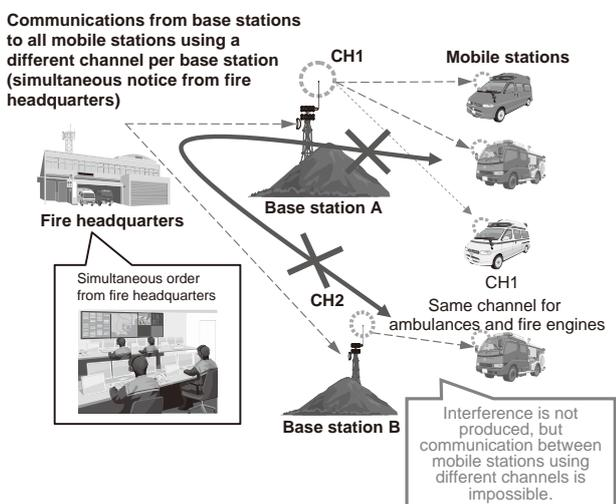
Fig. 4 Channel switching per base station.
