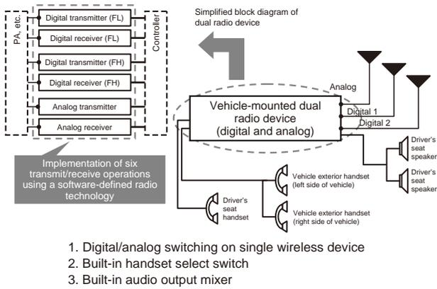
Fig. 11 Outline of a wireless communications system using a software-defined radio technology.
