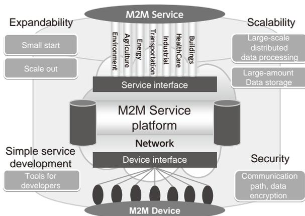
Fig. 2 CONNEXIVE M2M service platform.
