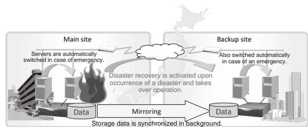
Fig. 3 Schematic diagram of disaster recovery system.
