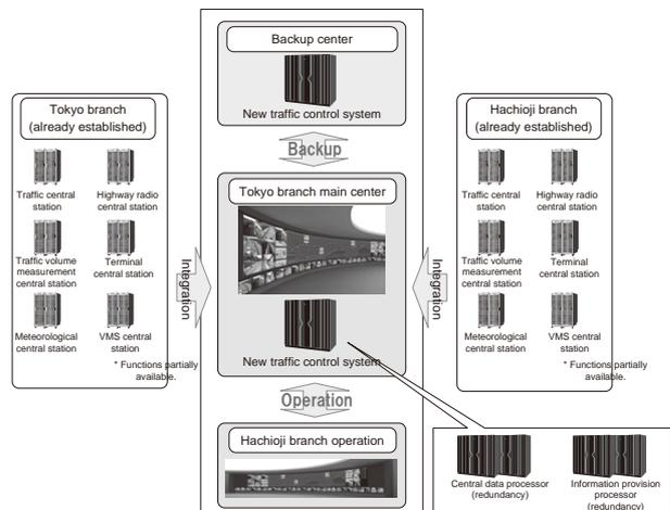
Fig. 2 Schematic diagram of the consolidation of equipment and functions.
