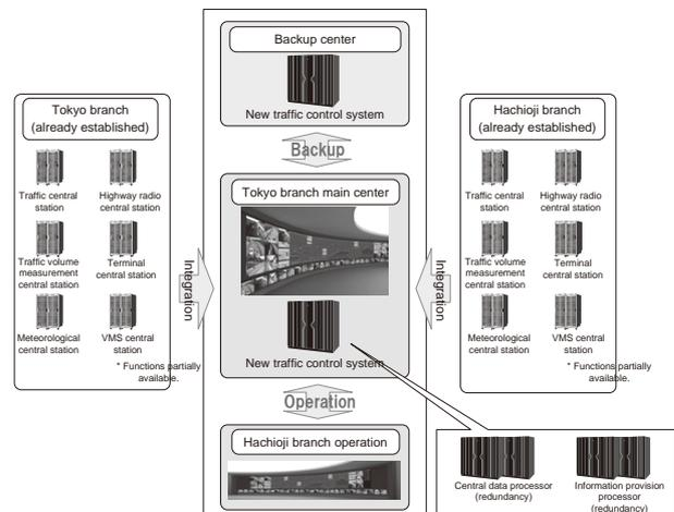
Fig. 2 Schematic diagram of the consolidation of equipment and functions.
