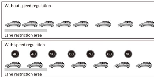
Fig. 4 Schematic diagram of traffic congestion elimination by speed regulation.
