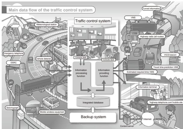
Fig. 1 Main data flow of the traffic control system.
