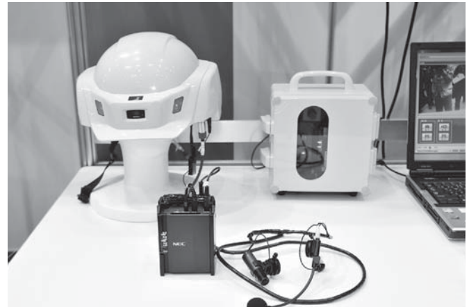
Photo 2 Field terminal for field visualization solution.
