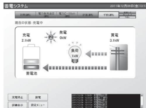
Fig. 3 Example of the system controller display.
