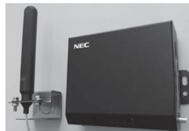
Photo 4 uM router incorporating various interfaces and functions.
