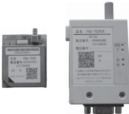
Photo 2 Embedded type module (left) and D-Sub 9-pin type module (right).
