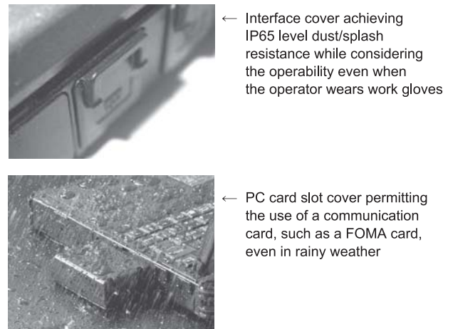
Fig. 4 Interface covers with improved dust/splash resistance.
