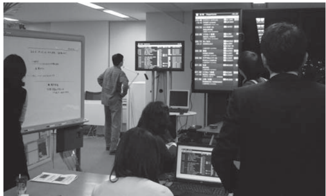
Photo 3 Visibility evaluations conducted on a prototyped display board of the same size as the actual display board.
