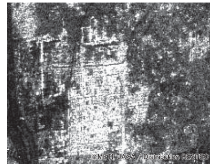
(b) Transmission with a polarized wave obtained by 60° rotation of vertical polarized wave/ Reception with a polarized wave obtained by 60° rotation of horizontal polarized wave
