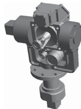
Fig. 5 Design results of SOTA's optics and acquisition/tracking mechanism.
