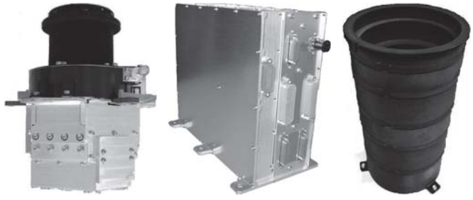
Photo 2 External view of a next-generation STT (From left to right: optical block, electrical block and baffle).
