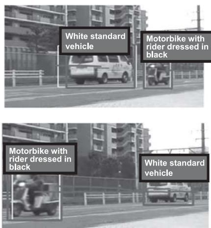
Fig. 5 Recognition and tracking of vehicles (Upper row: Initial. Lower row: Subsequent frame).
