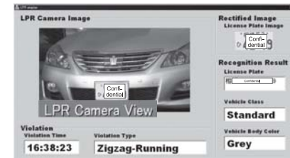
(b) Recognition of license number, class and color of meandering vehicle
