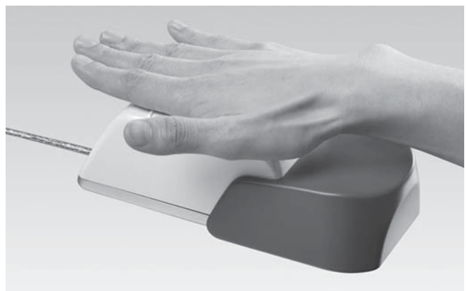
Photo 11 Palm recognition using a finger/palm hybrid recognition machine.
