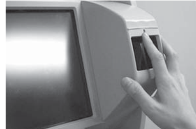
Photo 9 Hybrid scanner mounted in an automated teller machine.
