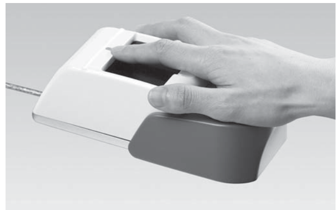
Photo 10 Finger recognition using finger/palm hybrid recognition machine.
