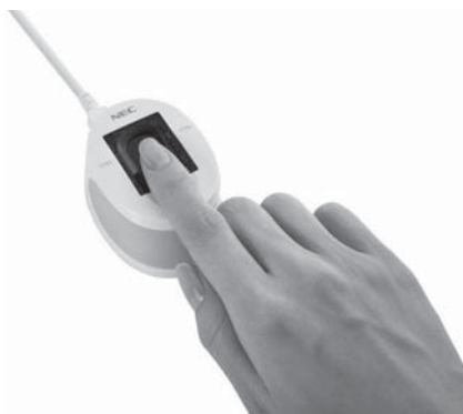
Photo PU900-10 fingerprint sensor with intra-finger scattered light scanning method.
