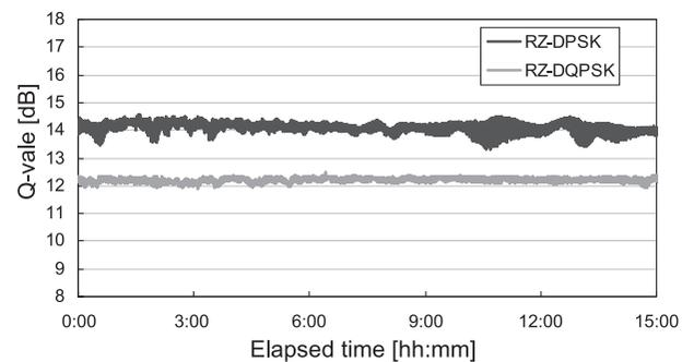
Fig. 5 Long-term stability after a 4,300-km transmission of 40 Gbps signals.
