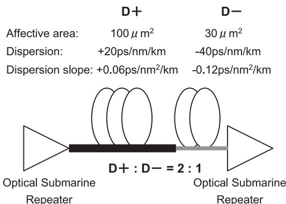
Fig. 1 Example of dispersion-managed fiber configuration.
