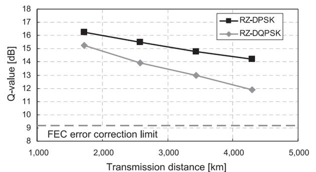
Fig. 4 Transmission distance versus Q-Value of 40-Gbps signals.
