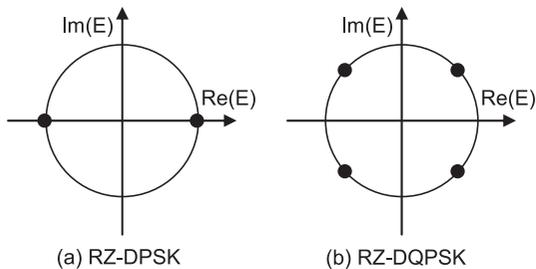
Fig. 3 Constellations of RZ-DPSK and RZ-DQPSK modulated signals.
