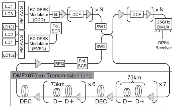
(a) 10-Gbps/132-wave transmission experiment setup
