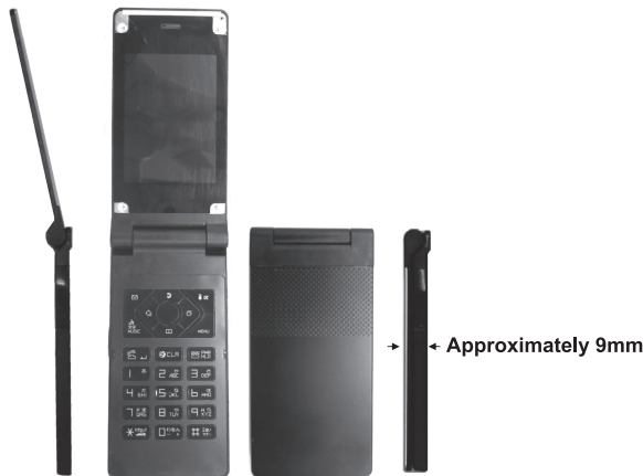
Photo Early prototype of the world-slimmest 3G flip-phone with a thickness of 9mm.
