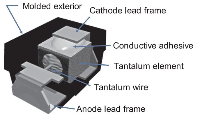
Fig. 1 Structure of NeoCapacitor.
