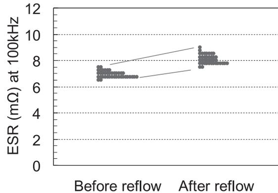
Fig. 3 ESR change of existing products before and after reflow.
