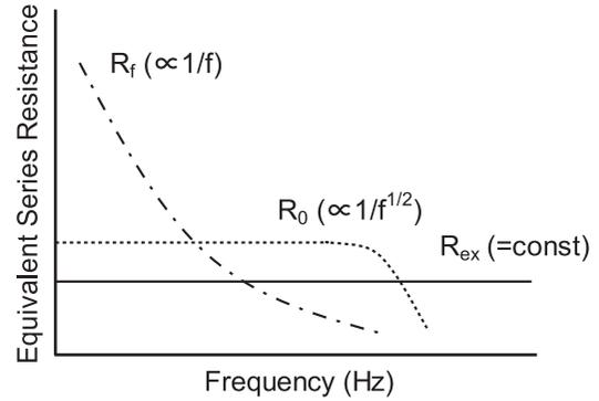
Fig. 2 ESR frequency characteristics.
