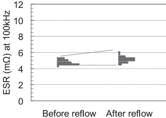
Fig. 5 ESR change during the production process of newly developed 6mΩ capacitors.
