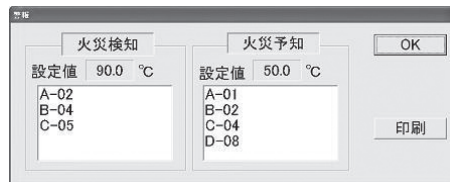
Fig. 5 Alarm display window.
