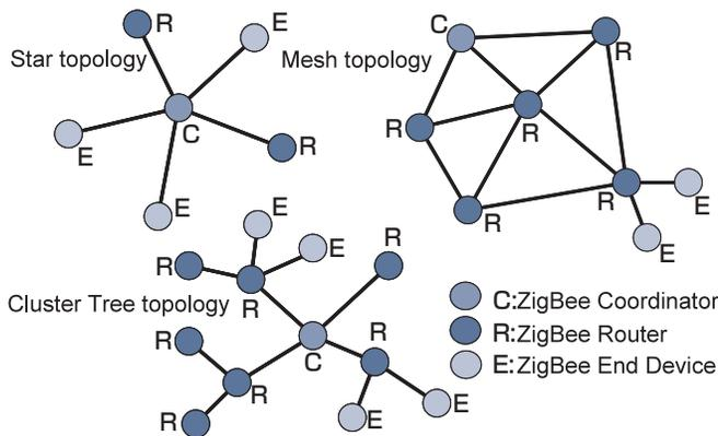
Fig. 2 Topology and 3 types of terminal functions.
