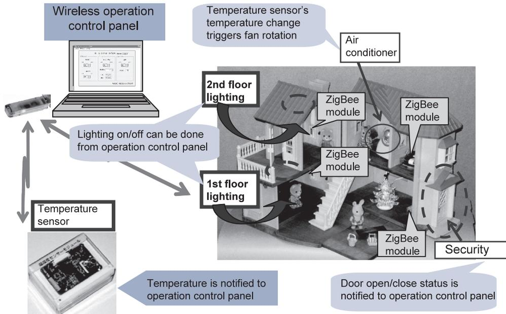
Fig. 4 A demonstration which simulates usage in the home.
