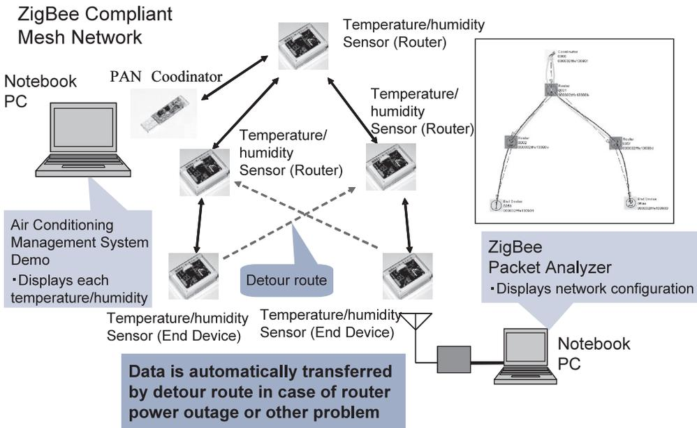
Fig. 5 Wireless temperature/humidity sensor network.
