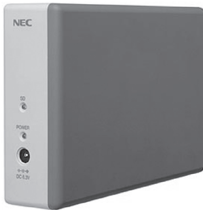
Photo 1 Wireless Gigabit Ethernet link product (a) for indoor use. Size: 200×50×140 mm 3 .
