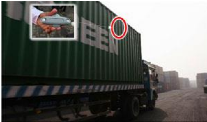
"RFID easily attachable to container using magnets"
