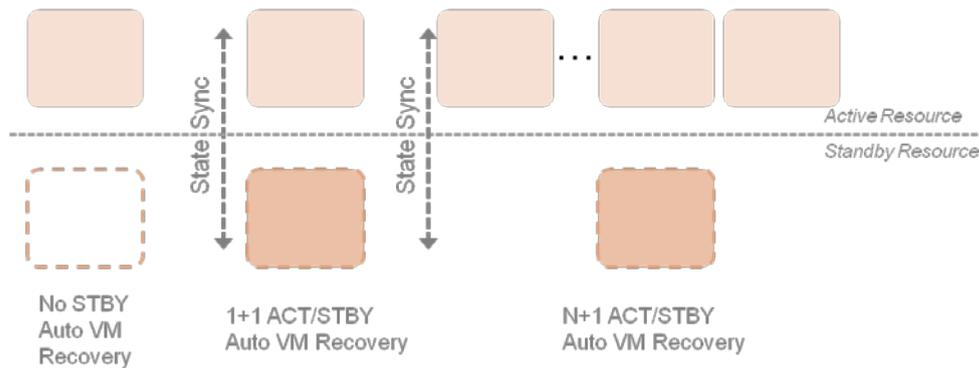
NEC vEPC’s redundancy, failover and VM recovery schemes meet carrier-grade requirements
