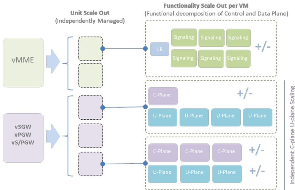
**NEC vEPC features an intelligent function decomposition that enables agility and elastic system scaling**
