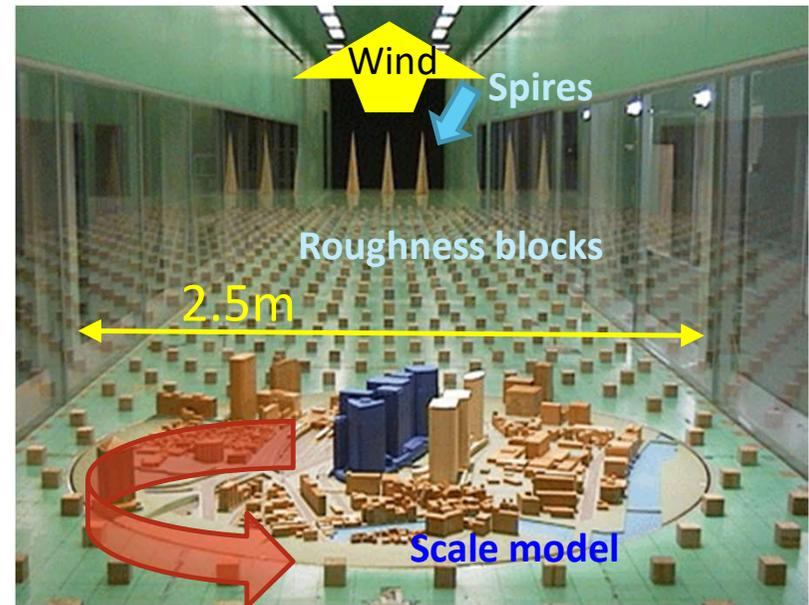
Wind direction : Rotating turning table (the angle of attack)
