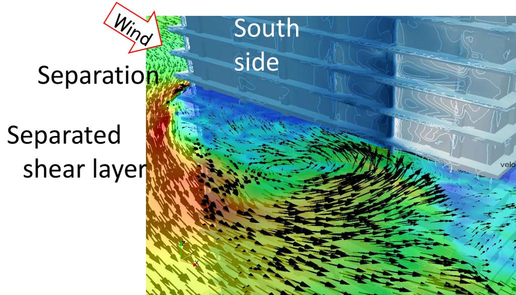
Fig. Horizontal flow field and pressure coef. distribution in the south side region of building
