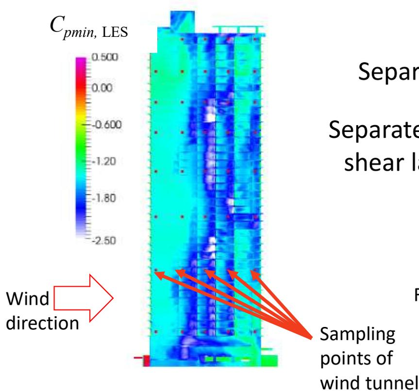
Fig. The min. pressure distribution on the south side.
