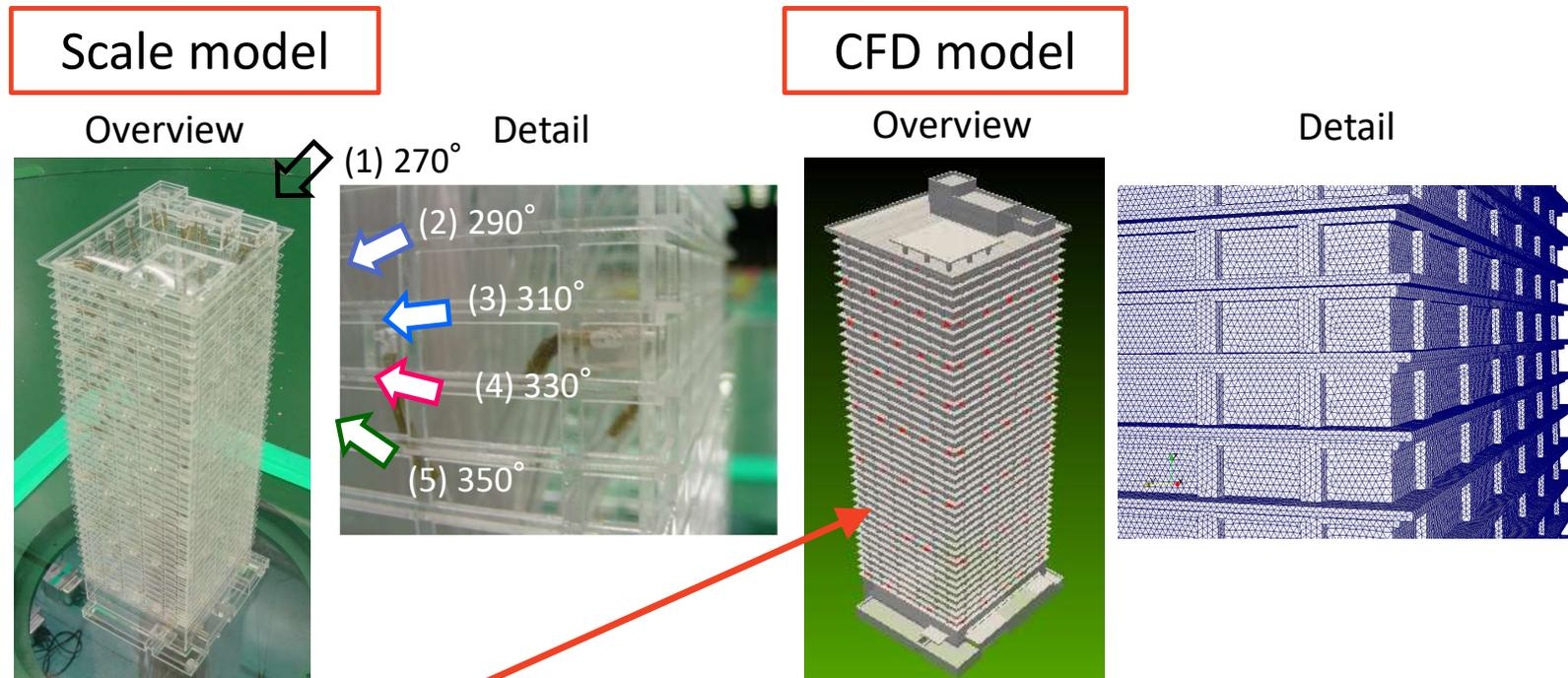
At every taps (**red points** in CFD overview), the experimental pressure values are obtained and compared with CFD.
