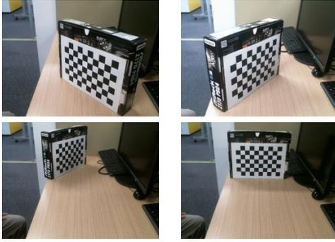
Fig. 5. Part of the images used for a comparison with a checkerboard calibration method. The image resolution is  $960 \times 720$ .
