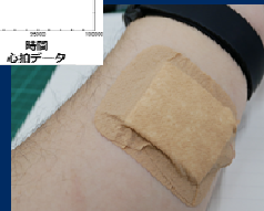
Accurate data can be collected by patch-type sensor without having an affection of body movements.
