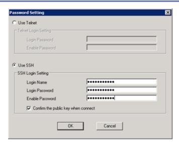
To use the SSH for connecting to the device.
