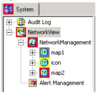
In the window shown above, for example, the event occurring in the "map2" node (FATAL, color-coded red) has higher priority than the "map1" node (UNMANAGED, monitoring mode OFF, color-coded gray), thus the "NetworkManagement" node, one level higher in the hierarchy, is displayed as FATAL severity level (color-coded red).
