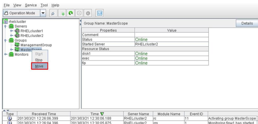
Figure 3-8 Switching between connected nodes
