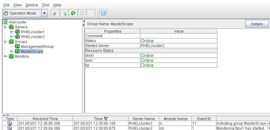
The screenshot displays the WebManager interface for a cluster. The left pane shows a tree view with 'rhelcluster' expanded to 'Groups', where 'MasterScope' is selected. The right pane shows the 'Group Name: MasterScope' configuration table. Below the table is an event log with the following data:
