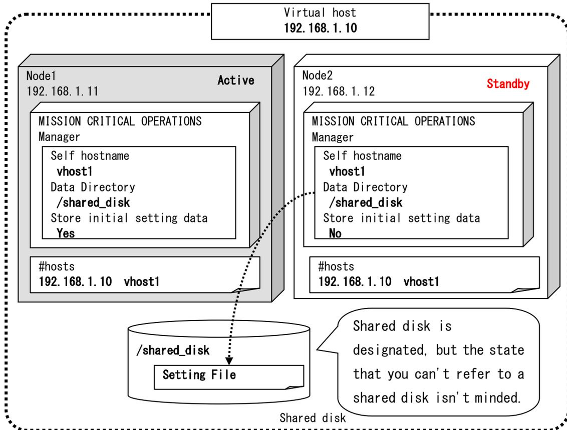
Specify each item in the installation setting dialog box for the MISSION CRITICAL OPERATIONS manager for the standby server node as shown below.
