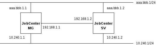
In the above figure, aaa.bbb.1.1 through aaa.bbb.1.2 are global addresses while 10.240.1.1 through 10.240.1.2, 192.168.1.1, and 192.168.1.2 are private addresses. Properly set up the network routing table so that jobs transferred from MG to SV and results returned from SV to MG go through the same network.
