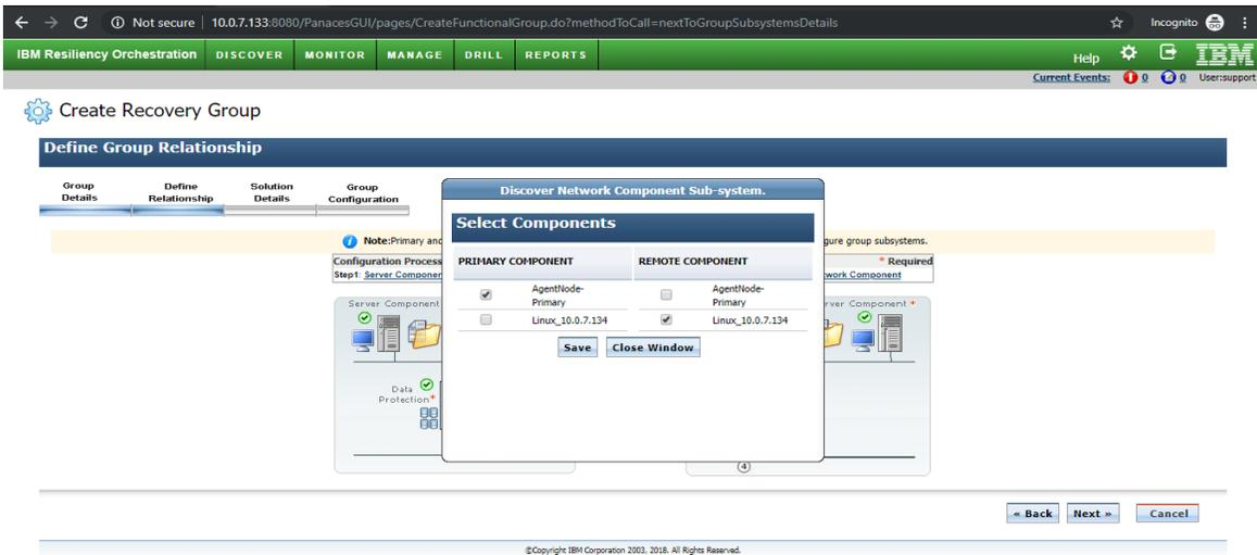
**Figure 21 Selecting Primary and Secondary Component**
