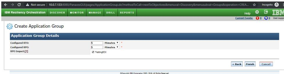
**Figure 31 Configuring RPO and RTO for the application**
