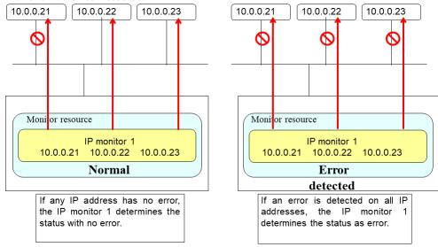
• If you want to establish error when any one of IP addresses has an error, create one IP monitor resource for each IP address.
