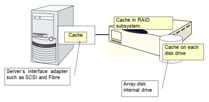
Note: This figure illustrates a typical example of shared disks. This is not applicable to all array units.
