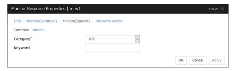
For **Category** and **Keyword**, specify a keyword passed using the -k parameter of the clprexec command. The keyword can be omitted.
